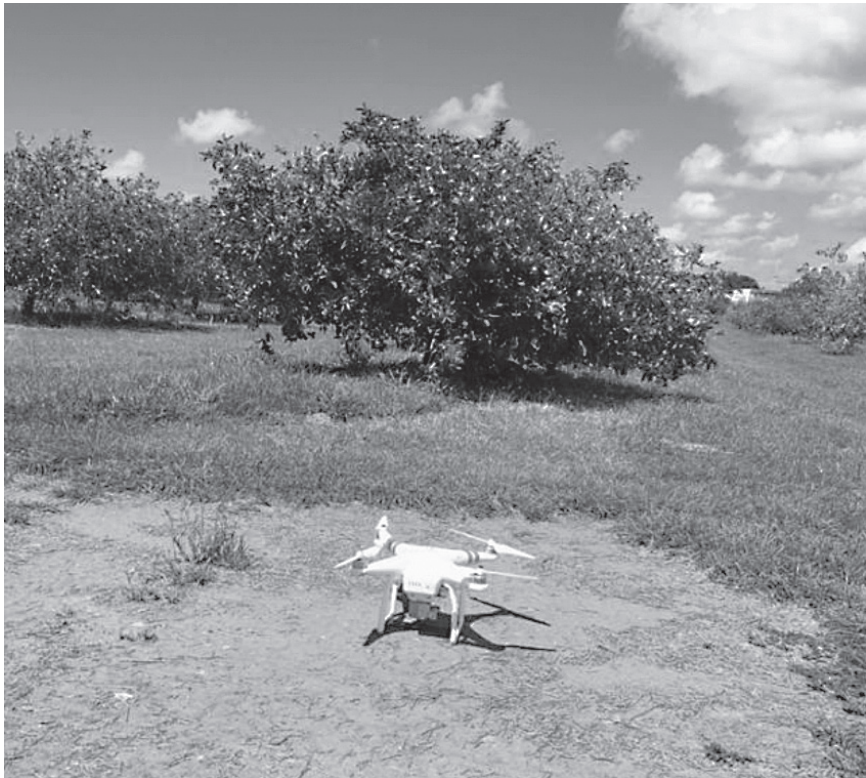
FIGURE 2. The unmanned aerial vehicle, DJI Phantom 3 Professional with 4K-color camera on board, used to acquire images of the citrus experiment.
