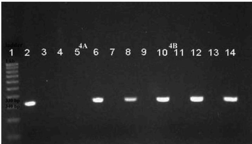
FIGURE 2. Agarose Gel of Polymerase Chain Reaction of Phakopsora spp. in Lablab purpureus . DNA amplification of ITS region of rDNA produced a 330 bp fragment observed with UV illumination after staining with ethidium bromide. Lane 1 = 100 bp ladder; lane 2 = Positive control for Phakopsora pachyrhizi (Ppa); lane 3 = Lablab Aibonito 1:10 Ppa; lane 4 = Lablab Aibonito 1:10 Phakopsora meibomiae (Pme); lane 5 = Lablab Aibonito 1:100 Ppa; lane 6 = Lablab Aibonito 1:100 Pme; lane 7 = Lablab Aibonito 1:1000 Ppa; lane 8 = Lablab Aibonito 1:1000 Pme; lane 9 = Lablab Corozal 1:10 Ppa; lane 10 = Lablab Corozal 1:10 Pme; lane 11 = Lablab Corozal 1:100 Ppa; lane 12 = Lablab Corozal 1:100 Pme; lane 13 = Lablab Corozal 1:1000 Ppa; lane 14 = Lablab Corozal 1:1000 Pme.
