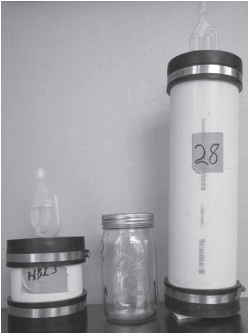
FIGURE 1. Laboratory mini-silos evaluated, from left to right: 1 L PVC, 1 L glass, 3 L PVC.
