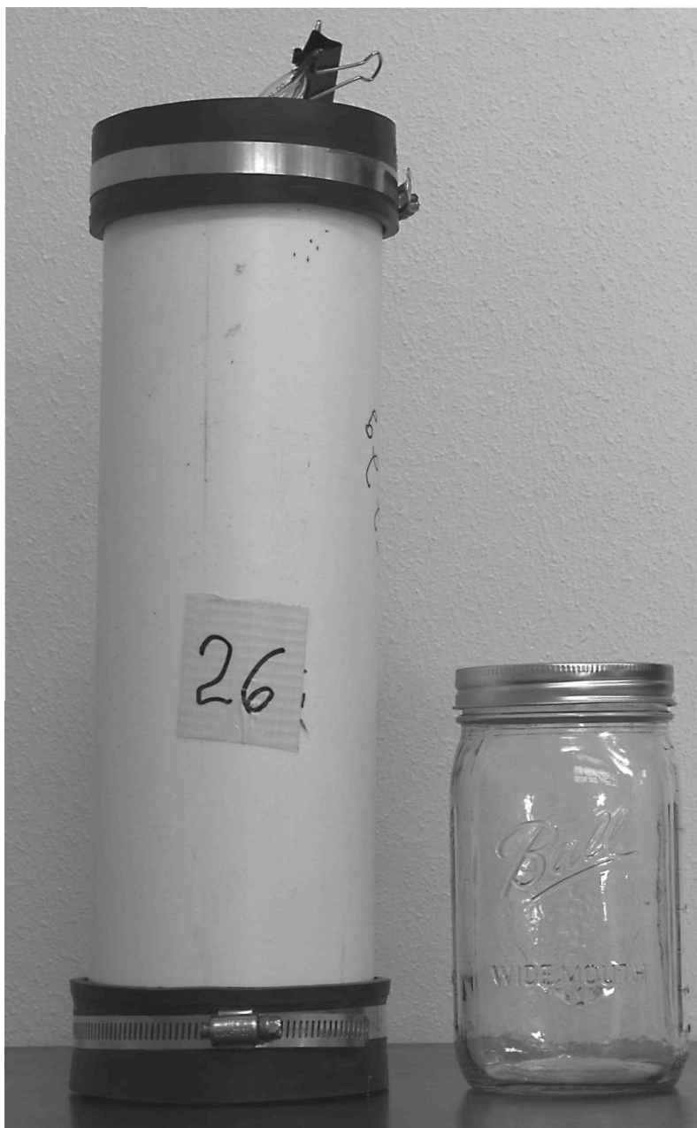
FIGURE 1. PVC and glass mini-silos used in Experiment #2.
