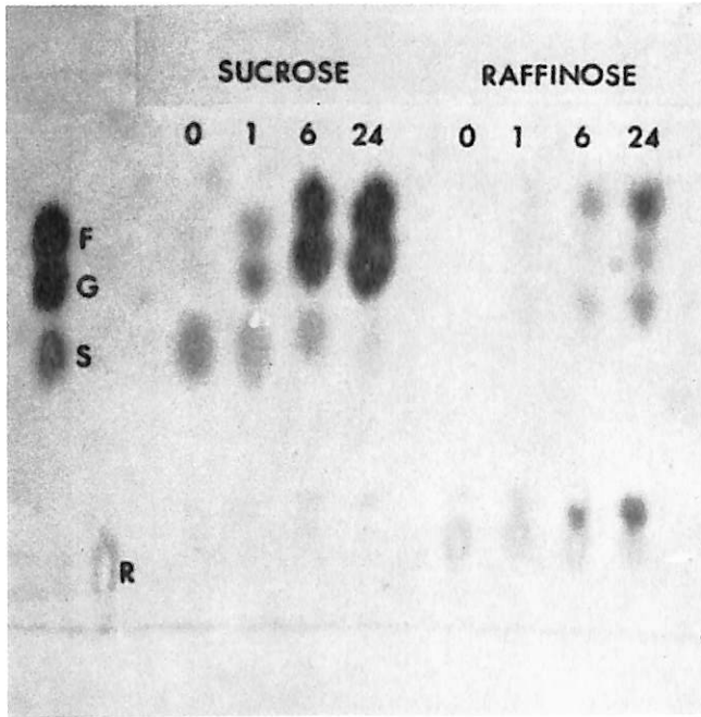
FIG. 2.—Action of sugarcane acid invertase on the substrates sucrose and raffinose over a prolonged period of time. The numerals 0 through 24 signify hours.
