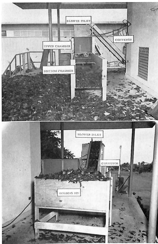
FIG. 1—End and side view of a single level arrangement for a coffee blower.
