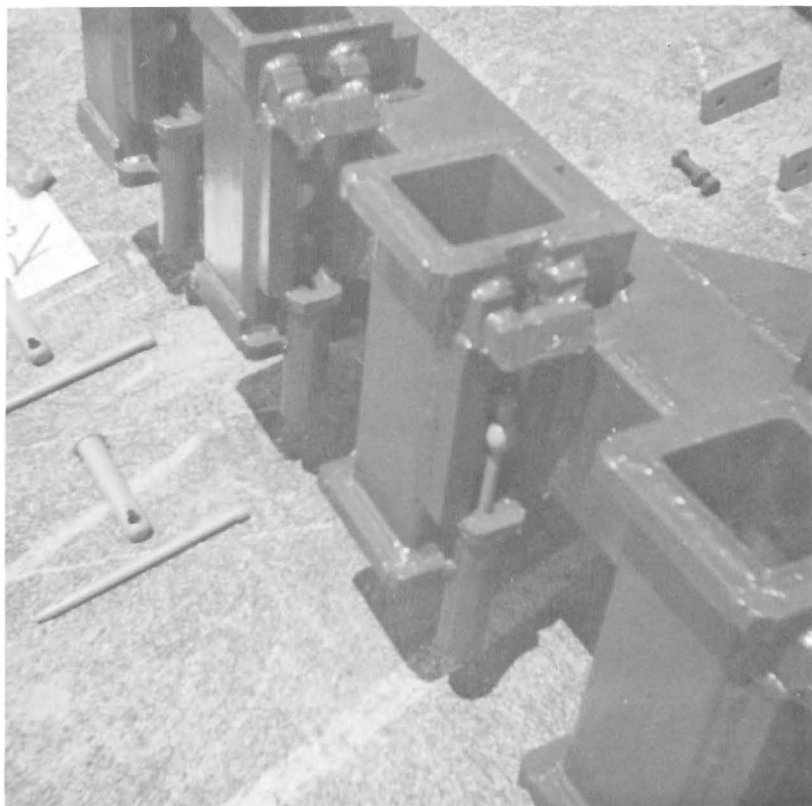
FIG. 5.—Close-up view of the holders showing the construction and components of the adjusting device.
