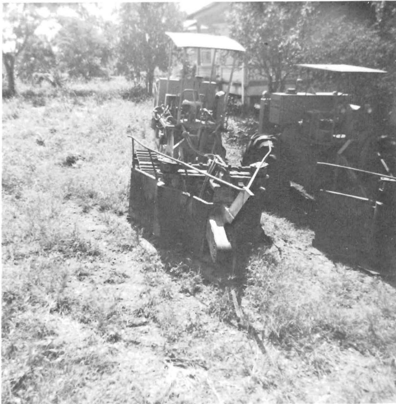
FIG. 3.—View of the V-cutter popularly known in Puerto Rico by the name of "La Coneja".
