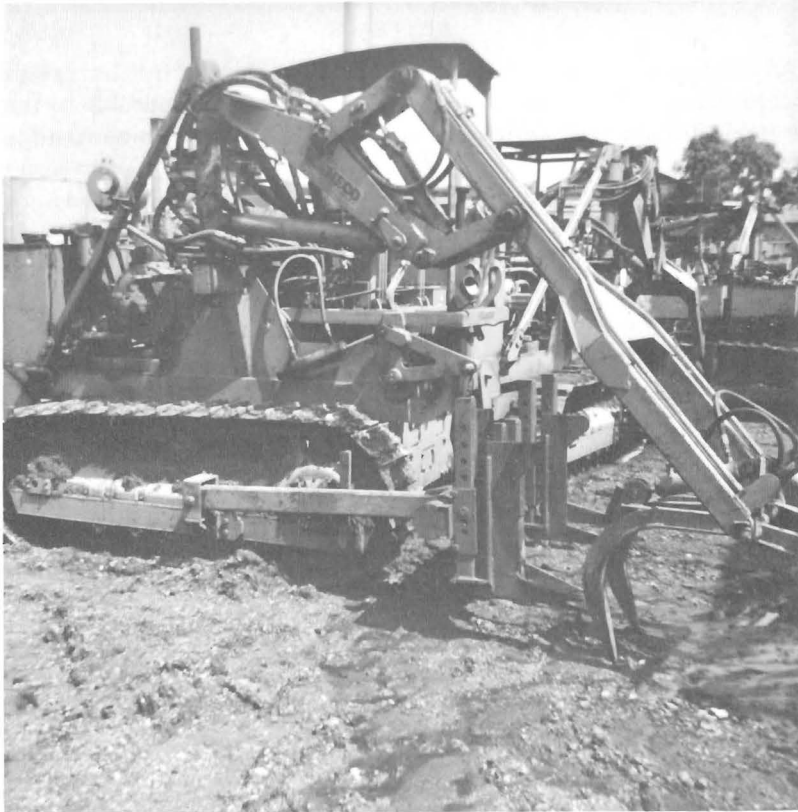
FIG. 6.—The adjustable sugarcane piler mounted on a track-type loader.
