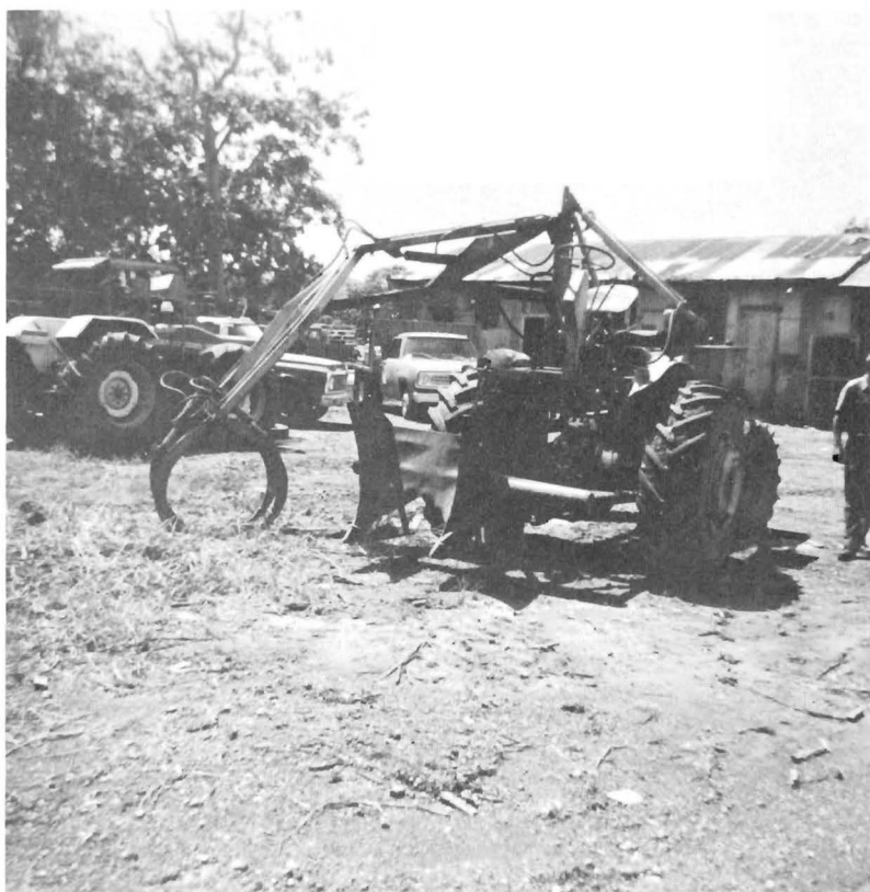
FIG. 2.—A conventional 2-pointed piler as currently used with hand-cut and manually windrowed cane.
