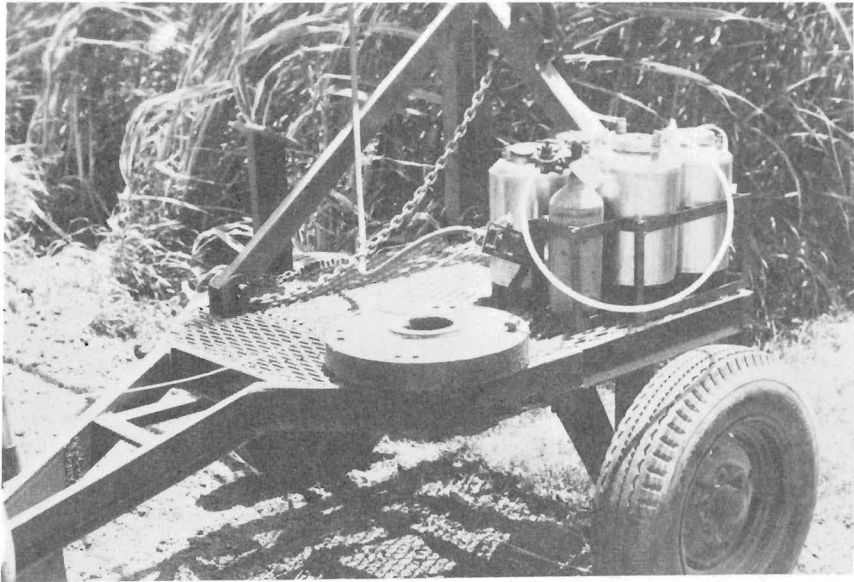
FIG. 2.—The 2-wheel carrier and rear-mounted square mast.
