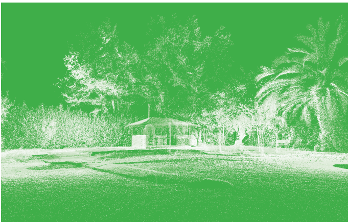
Figure 1. View of the site after digitally removing the previous construction to start the design, rendered from the 3D laser scanning.
